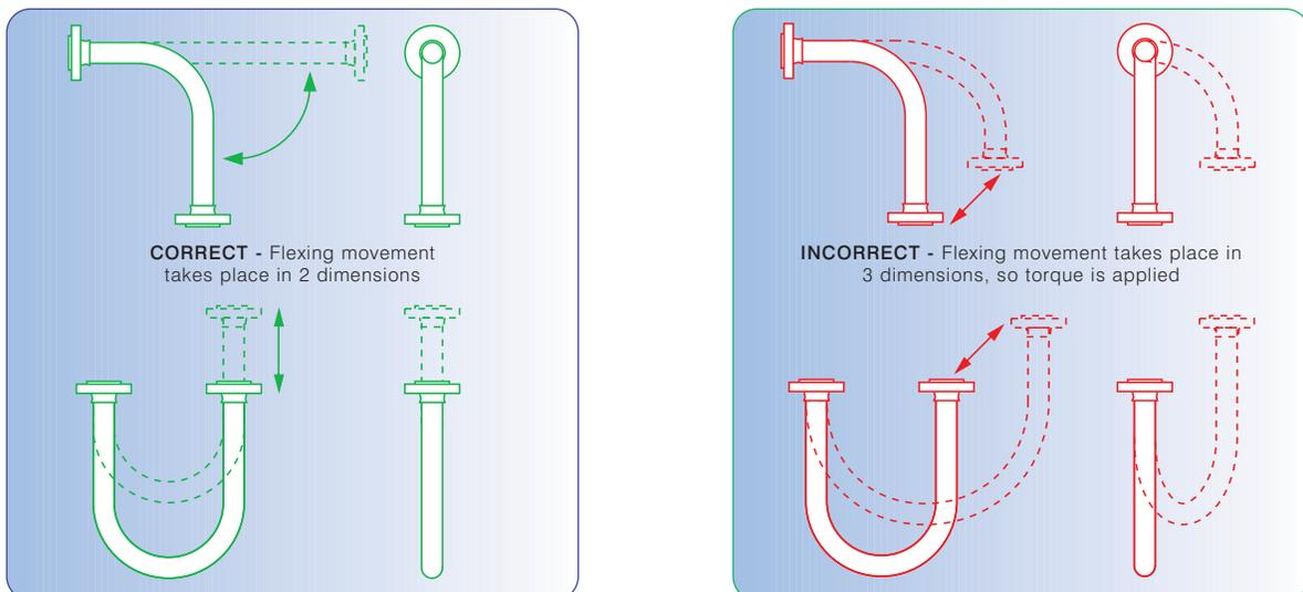
Both Corroflon and Bioflex hose have good resistance to a small level of torque, much better resistance than rubber or SS hose types, but it is still the best practice to take whatever steps are necessary to eliminate torque. If in doubt, consult Aflex Hose.
